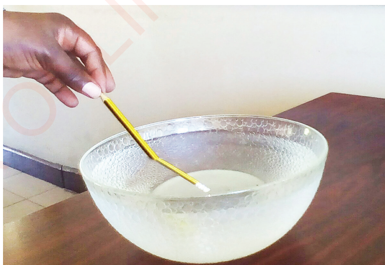
Figure 14: A pencil immersed in water to show the effect of bending of light rays
